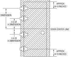
FIGURE 3 illustrates a typical door/jamb where SOSS Invisible Hinges will be mounted. Become familiar with the terminology as it will be used throughout these instructions.
