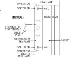
**4** REFER TO TABLE "A" to obtain the proper size drill or spade bit and starter hole depth.
