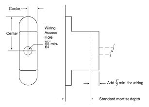
Install top and bottom SOSS® Invisible Hinges to support the door on the frame.
