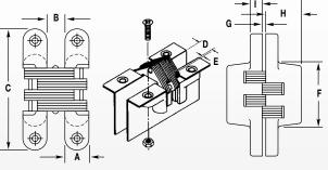
All metal cabinet hinges are shipped without screws unless otherwise specified. **Do not exceed "E" dimension.**
