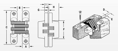
All fire rated hinges are shipped with the proper size wood and machine screws unless ordered without. Do not exceed "E" dimension.
