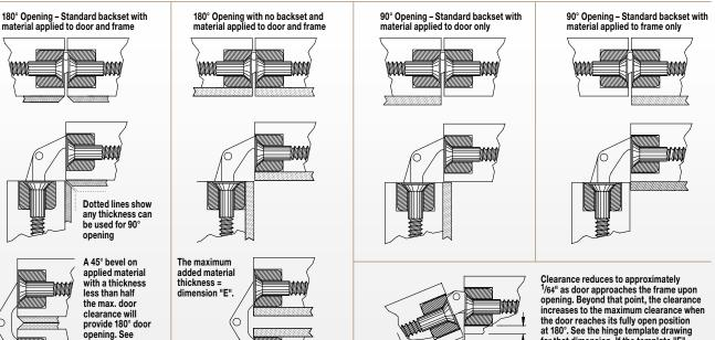
increases to the maximum clearance when the door reaches its fully open position at 180°. See the hinge template drawing for that dimension. If the template "E" dimension is exceeded, the door will hit the jamb and bind. See specifications for SOSS Invisible Hinges on previous pages for dimension "E".
