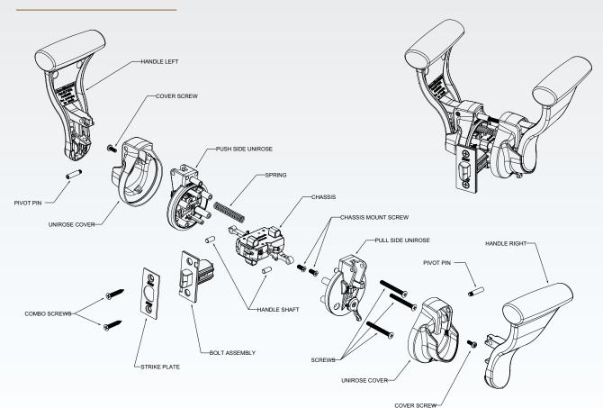
When you receive your UltraLatch from the factory, it will be ready for installation into a left hand door. Instructions are provided with the UltraLatch for changing the assembly to fit a right hand door.
