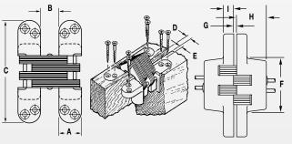
All power transfer hinges are shipped with the proper size wood and machine screws unless ordered without. **Do not exceed "E" dimension.**
