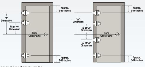
For small cabinet doors using the light or medium duty hinges the spacing for the top and bottom hinges need only be 2- 4 inches from the top or bottom of the door to the center line of the top or bottom hinge respectively.
