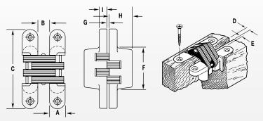
All hinges are shipped with the proper size wood screws unless ordered without. Machine screws available upon request for an additional charge. Do not exceed "E" dimension.
