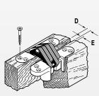
All SOSS Hercules Hinges are shipped with the proper size wood and machine screws unless ordered without. **Do not exceed "E" dimension.**
